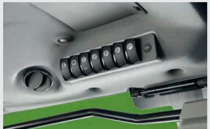
↑ Protection against pesticide aerosols, given by Cat.4 filtration, can be easily activated through a button.
