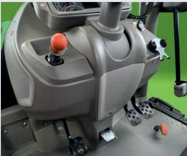
↑ Equipped with all-wheel braking and a Hydraulic Parking Brake (HPB) as standard.
