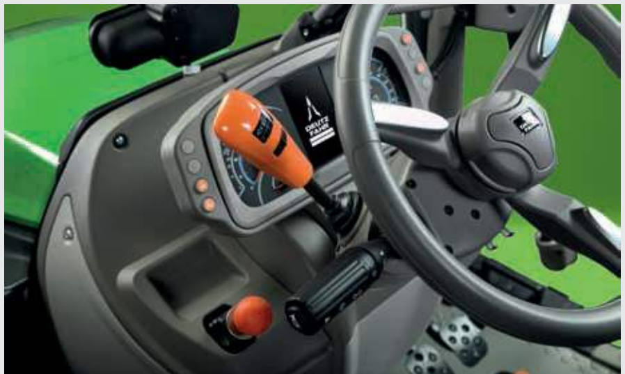
↑ PowerShuttle with SenseClutch (5 adjustable levels).
