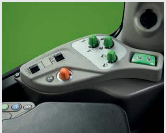
↑ The driver can select within a range from "ECO" engine management mode to "Power", for maximum power.
