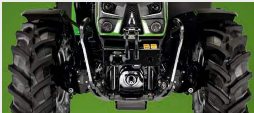
↑ 5D TTV models can be equipped with a front lift with 2,100 kg capacity and optional comfort package.
