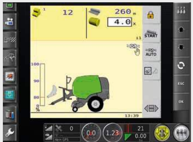
↑ Universal Terminal to control any ISOBUS implement.
