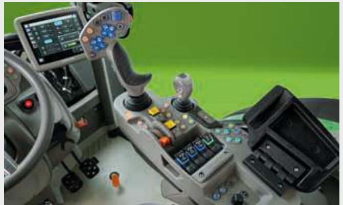
↑ MaxCom armrest with intuitive color-coding for easy handling.
