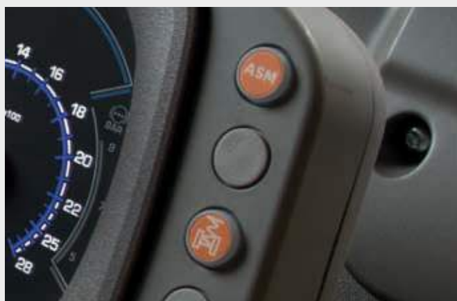
↑ ASM and front axle suspension activation.
