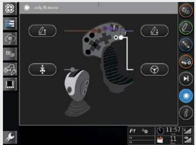
↑ 3 jolly buttons and 1 programmable thumbwheel.
