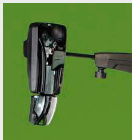
↑ Mirrors with electric adjustment and defrosting.
