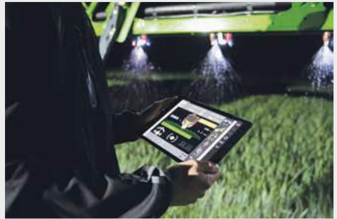
↑ XTEND function, control of implements with ISOBUS UT via tablet while being outside of the cabin.
