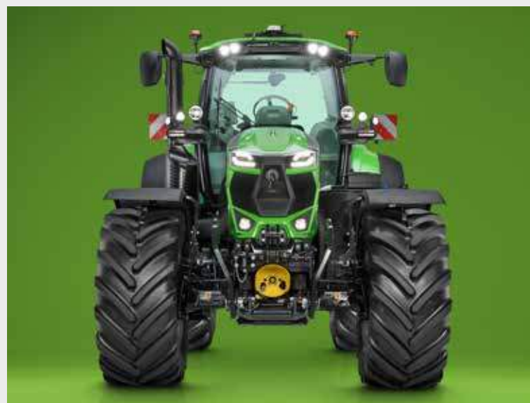
↑ The DualSpeed front PTO offers a splined stub shaft which is removable, allowing the tractor to be connected to implements with drive shafts of any type.
