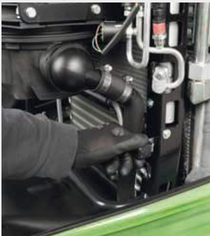
↑ Cooling package with easy opening mechanism.
