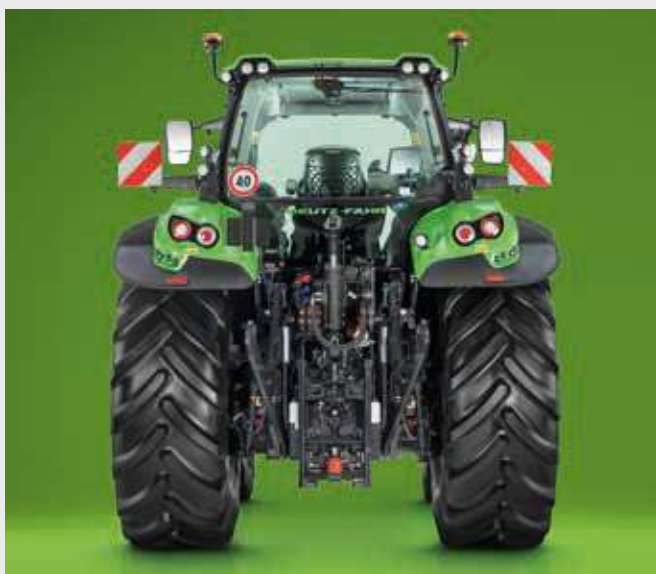
↑ The "Clean Oil System" delivers up to 90 litres of oil to the implements and ensures lowest maintenance cost thanks to 2000 h or 2 years change intervals.
