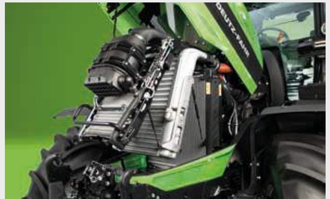
Aluminium cooling system of 6210 TTV, 6230 TTV and 6230 TTV HD with one-hand access lever and Powercore air filter.
