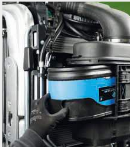
↑ Airfilter with pre-cleaning unit.
