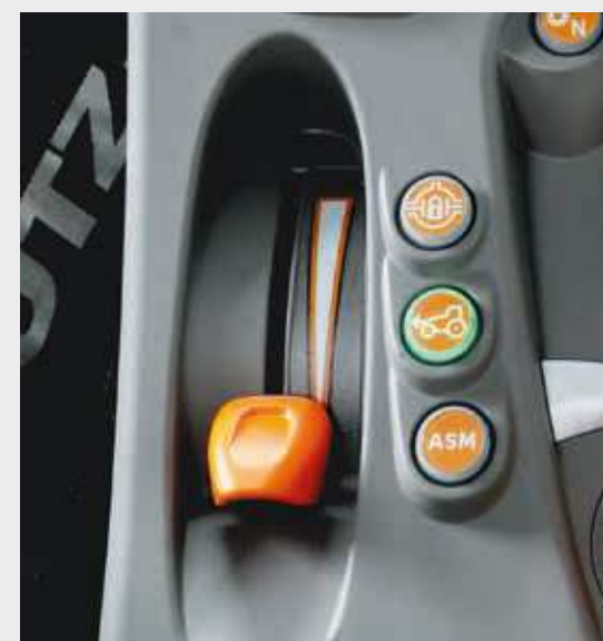
Independent hand throttle and electrohydraulic activation of differential lock, four-wheel drive and ASM function.
