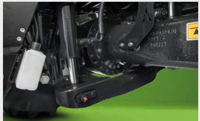
↑ Front axle of 6190 TTV with a robust lower swing arm.
