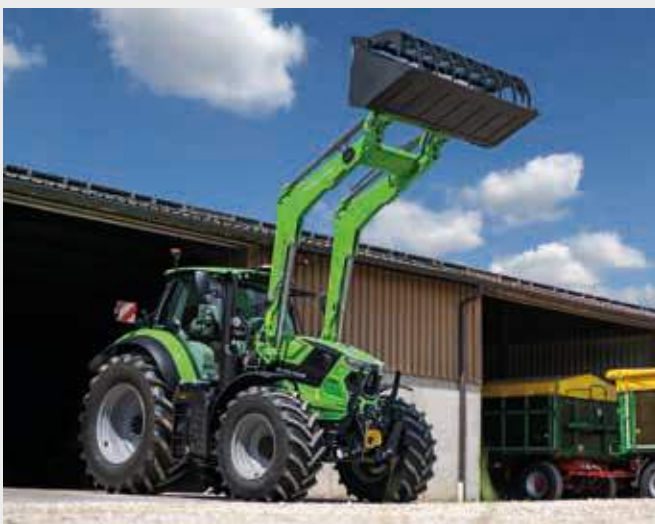
↑ Maximum lifting height of 4.5 m and a breakout force of 3770 daN.
