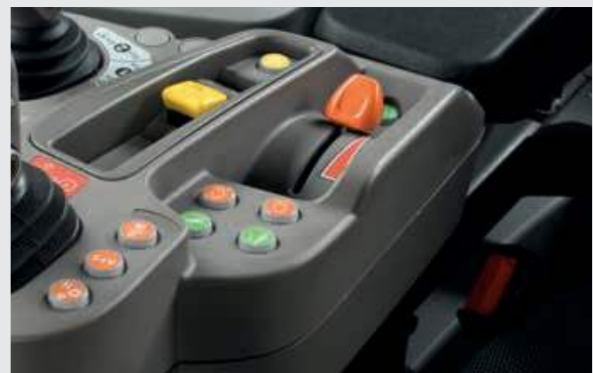
Electronic hand throttle with 2 engine memory speeds.
