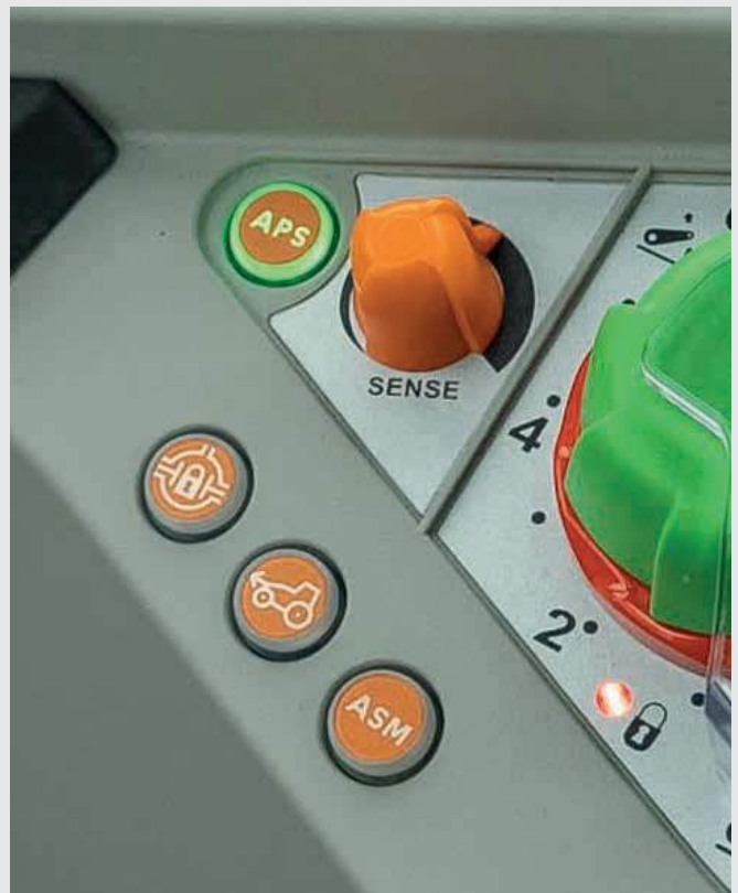
APS activation with adjustable response.
