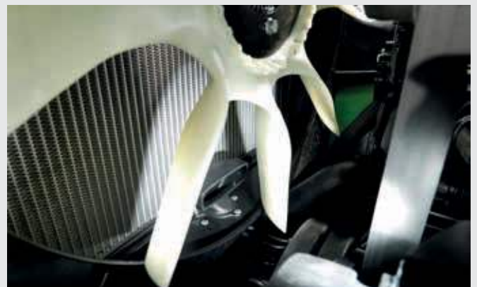
↑ Electronic viscous fan (eVisco) with suction hose for air filter pre-cleaning system.
