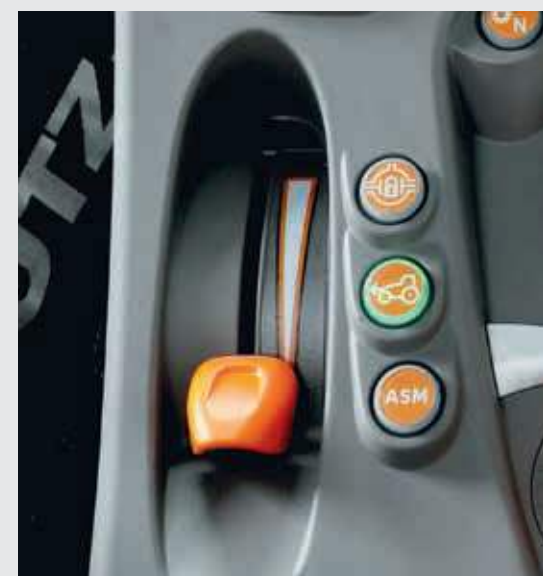
↑ Independent hand throttle and electrohydraulic activation of differential lock, all-wheel drive and ASM automatic function.
