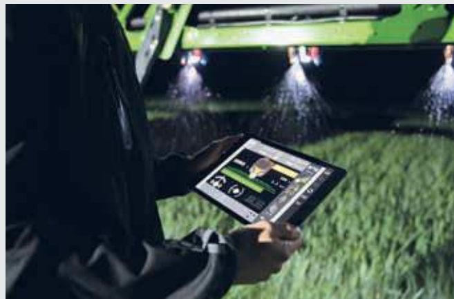
↑ XTEND function with tablet, control of implements via ISOBUS UT while being outside of the cabin.
