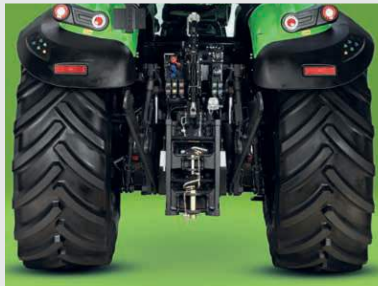
Rear linkage, five rear spool valves, external controls on fenders on both sides.
