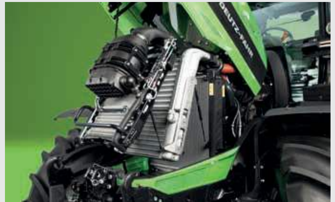
↑ Aluminium cooling system with with one-hand access lever and Powercore air filter.
