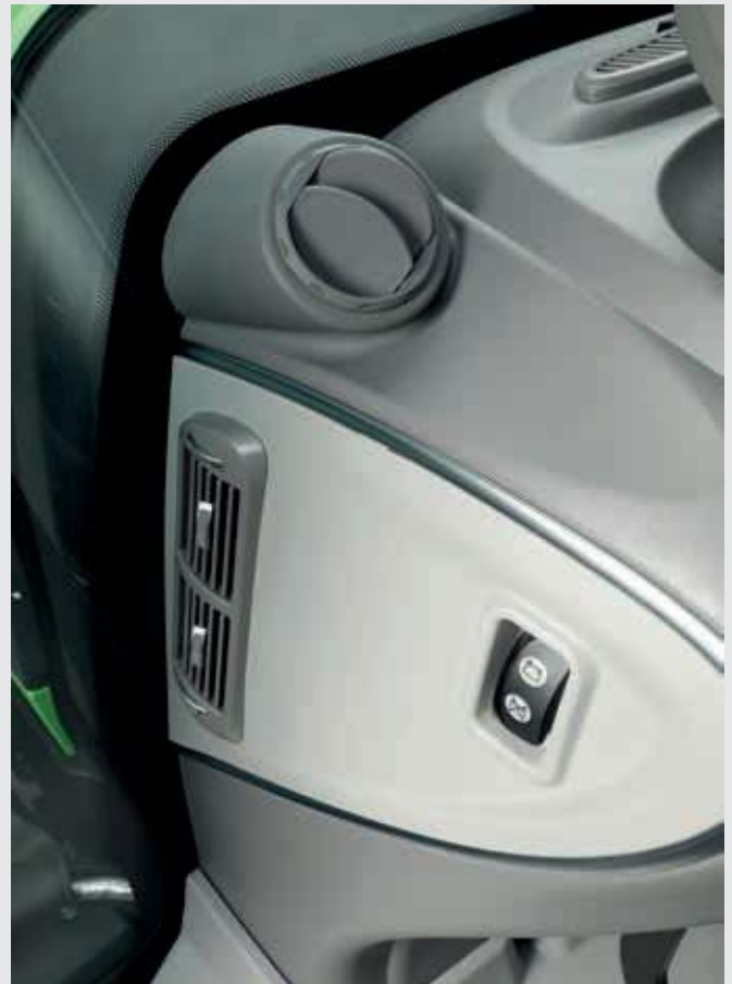
Additional air outlets and battery main switch comfortably placed in the cabin.
