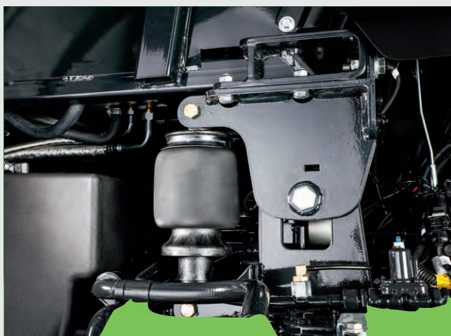
↑ Pneumatic cab suspension for a smoothest ride.
