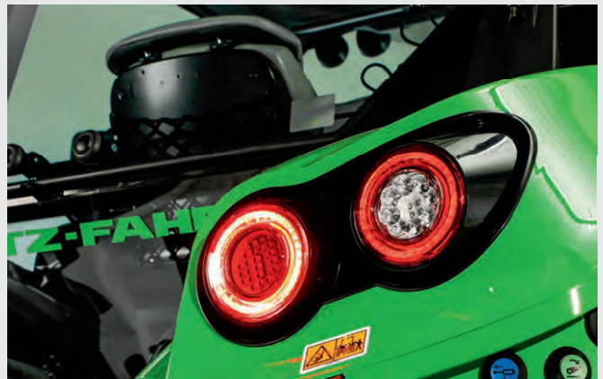
↑ LED turning indicator available for more safety and nice and modern appearance.
