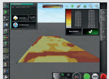
↑ The TC-Geo can be used to process e.g. application maps. This is already standard in the 12" monitor.
