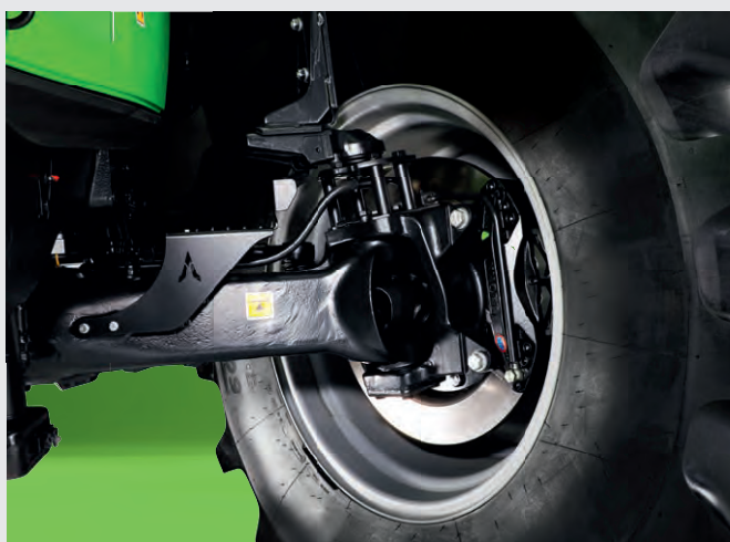
↑ Dry disc brakes for maximum brake performance.
