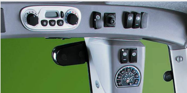
Driving lights, work lights and cab lights all on one control panel. Select the work climate and the automatic function control the air flow.
