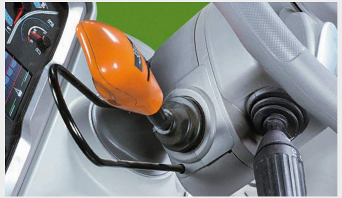
↑ Standard: Powershuttle system. The sensitivity (hard – medium – soft) can be easily adjusted with a thumb control.
