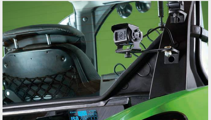
↑ Integrated camera with automatic full screen mode (e.g. reversing) for overview and safety.
