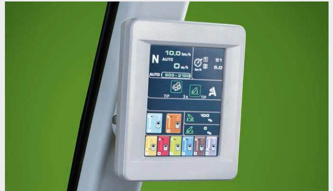
↑ Three driving/work strategies can be selected: manual, automatic and PTO. These are displayed on the WorkMonitor.
