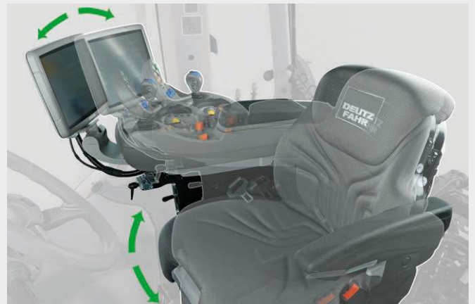
Now available for all TTV models: Seat with up to 20° rotation for added comfort and ease of operation.
