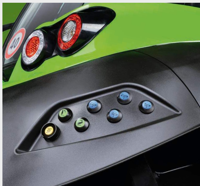
↑ External control of the hydraulics and PTO functions from either side.
