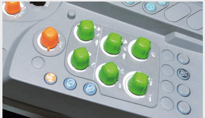
↑ ... as are the front and rear linkage controls.
