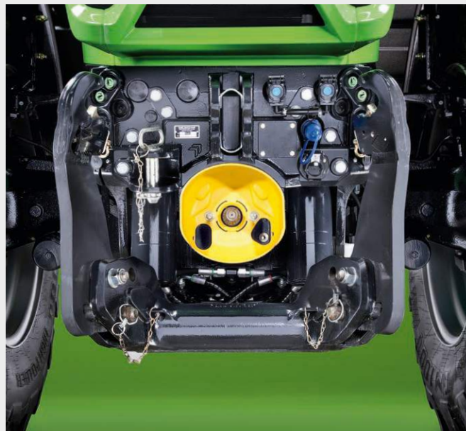
↑ Integrated front linkage with uniquely short distance to the front axle. Low overhang. Best tractor balance.
