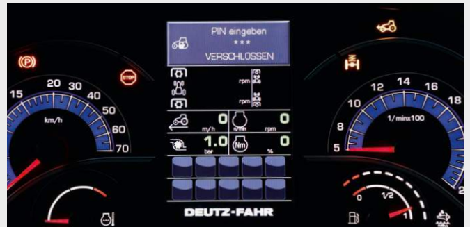
The new InfoCenter keeps the driver up to date: analogue and digital information about the operating status. Safety thanks to the code lock for the tractor. Lock and unlock with a PIN.
