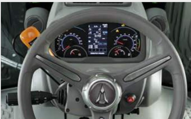
↑ State-of-the-art dashboard with InfoCentre Pro : 5" high-resolution display. The iLock function enables lock and unlock with a PIN.
