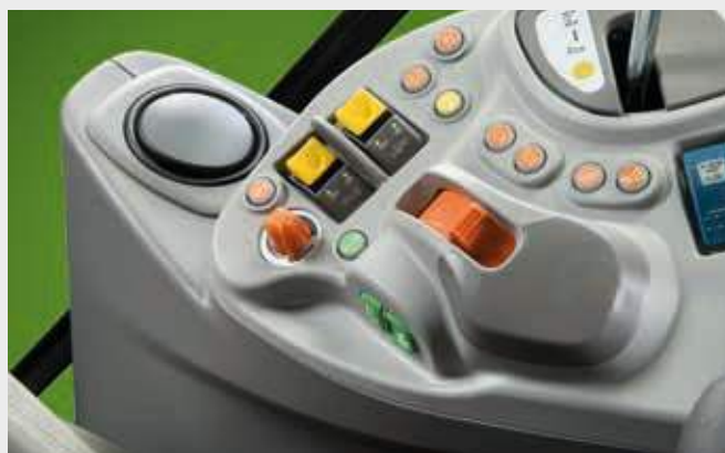
↑ Front and rear PTO electrohydraulically engaged and AUTO PTO function.
