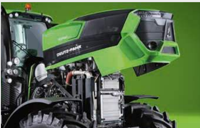
↑ An electrically opening hood facilitates maintenance work.
