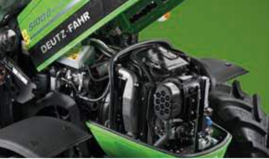
↑ Compact radiator with Visco fan and PowerCore air filter for maximum engine efficiency.
