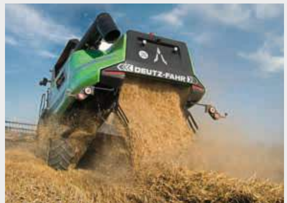
↑ Best material flow thanks to the open straw-hood.
