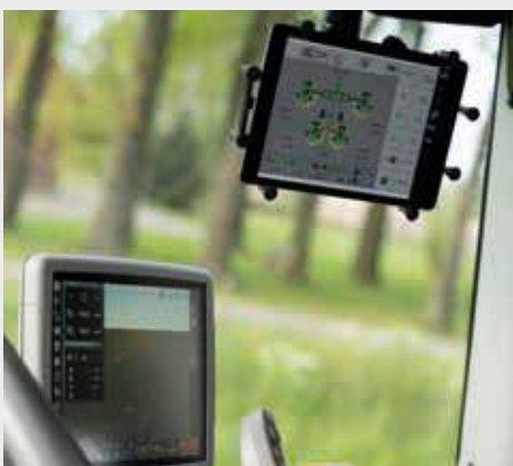
↑ XTEND allows to show on a tablet SDF Guidance or let you control an ISOBUS implement.
