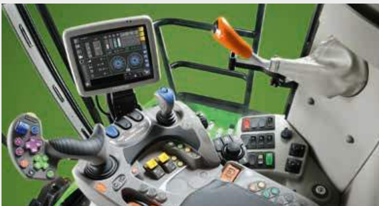
↑ With the ergonomic armrest integrating the COMMANDER STICK and the iMonitor you can perform all combine harvester adjustments in a simple and effortless manner.
