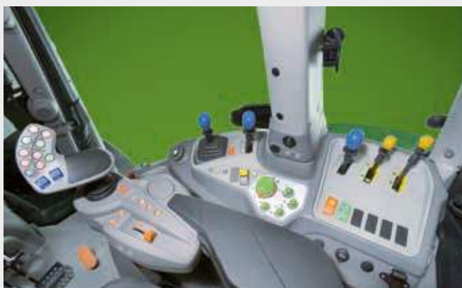
RCshift transmission: MaxCom Joystick always included.
