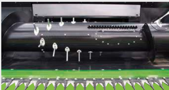
↑ Large diameter of the intake auger with adjustable fingers in spiral all along the entire cutting width.
