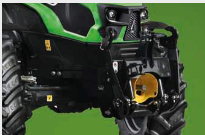
⬆ On request, the 5D models can be equipped with front linkage and front PTO.
