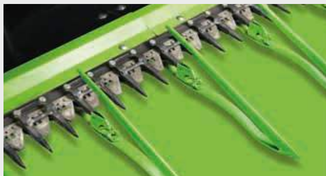
↑ Standard crop lifter easy-to-mount and special guide rollers (optional) reduce vibration and wear even further.
