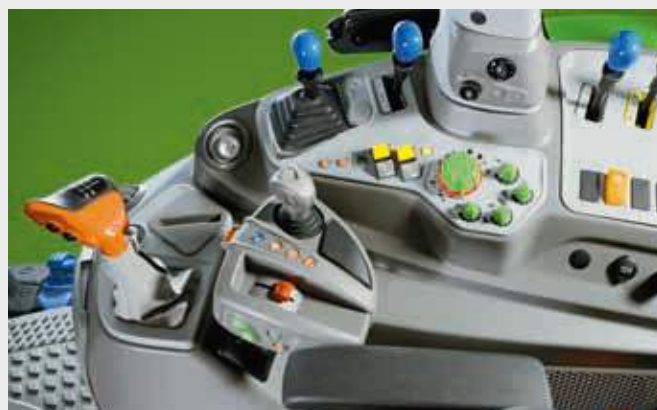
Powershift transmission: efficient all-round transmission with manual gear lever.
