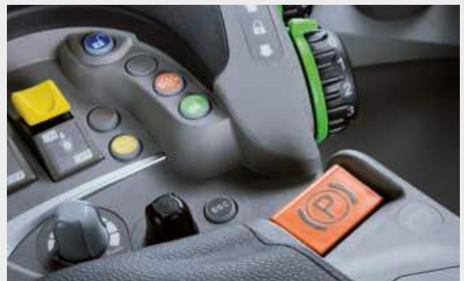
↑ Electronic Parking Brake (EPB) integrated into MaxCom armrest.
