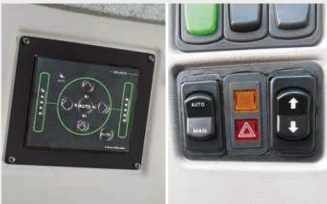
↑ Independent control between front BALANCE and rear levelling system, both with automatic or manual function.
