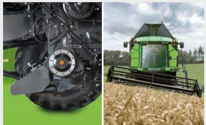
↑ The 25 t capacity axles allow the machine to work in the most extreme conditions, ensuring utmost reliability and, above all, driver safety.
