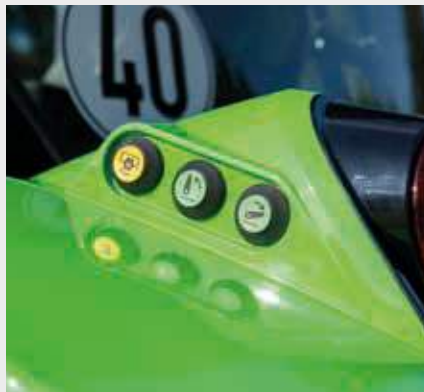
↑ External controls for rear lift and PTO.
