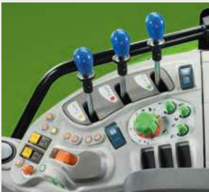
↑ Ergonomic layout of rear lift controls and hydraulics levers.
