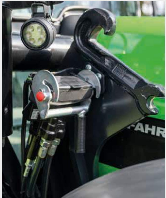
Front loader fixed frame with Hydro-Fix connection.
